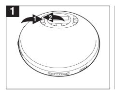
During playback, depress and hold either the Skip/TUNING DN IM ① or UP IM ② button to move the player forward or backward within a track to locate a specific musical passage. The player will move forward or backward at high speed as long as the buttons are depressed. When you release the Skip/TUNING DN IM ② or UP IM ② button, normal playback will resume.
