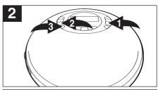
Within ten seconds, select the desired preset using the PRESET UP  $\blacktriangle$  ① or DN  $\blacktriangledown$  ② button to set the memory. Press the PROG. button ③ to confirm.
